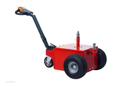
Tighten all wheel bolts to 120nm after the first 2 hours of driving.
